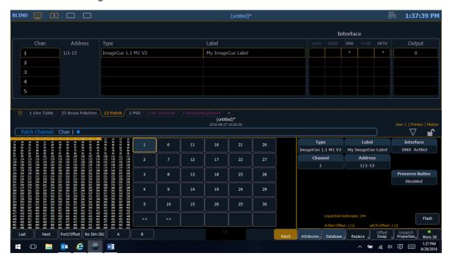
7. Once the fixture is patched, select it (Channel 1 in the example). The ML Controls (moving light) screen will provide access to all of the parameters at one time:
