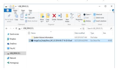
3. Insert the USB Drive into the console. Start the console or Nomad. You can add the profile to an existing show, or start with a new show. The screen shots shown are for a new show. In "LIVE" mode, open the Browser.
